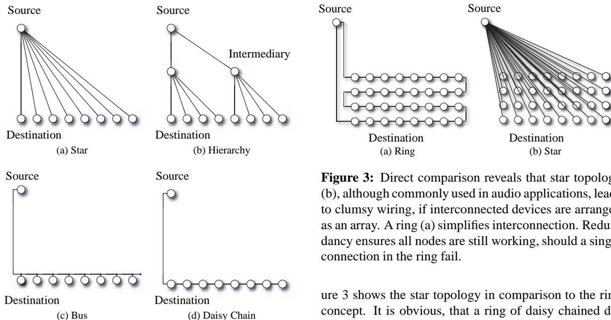
**Figure 2:** Common types of device connections for signal distribution from a single source to multiple destinations.
