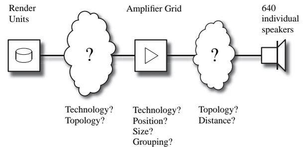
**Figure 1:** The tasks to be considered in the design of a massive multichannel loudspeaker system.
