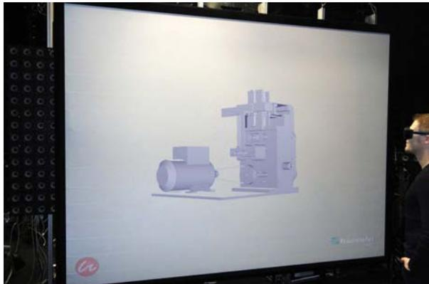
**Figure 9:** Use of the loudspeaker wall in combination with stereoscopic video projection. The images shows the visualization of a pick & place unit that is continuously rotated around the vertical axis. The render units that drive the loudspeakers behind the perforated screen generate signals for the auralisation of the directional sound field of the example machine.
