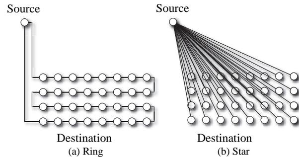
**Figure 3:** Direct comparison reveals that star topology (b), although commonly used in audio applications, leads to clumsy wiring, if interconnected devices are arranged as an array. A ring (a) simplifies interconnection. Redundancy ensures all nodes are still working, should a single connection in the ring fail.
