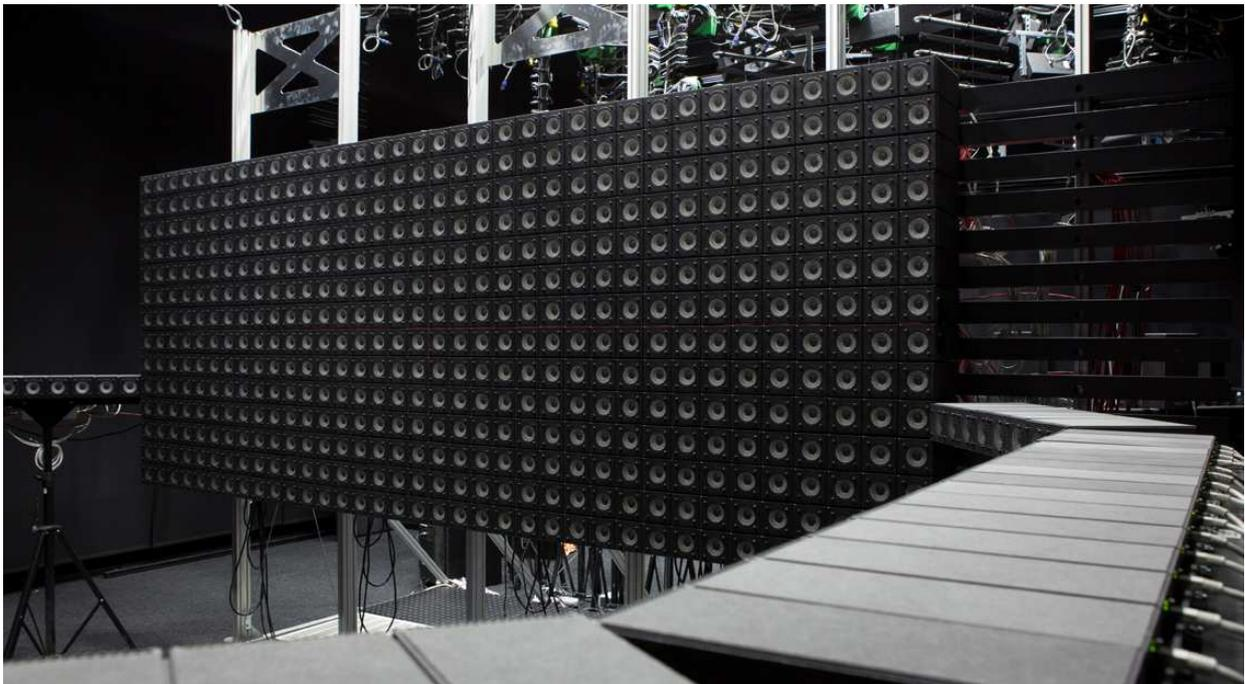
**Figure 4:** Image of the multichannel loudspeaker system, installed in the special acoustical laboratory at Fraunhofer. The system consists of 504 loudspeakers stacked as a wall and a surrounding circular array consisting of 100 loudspeakers.
