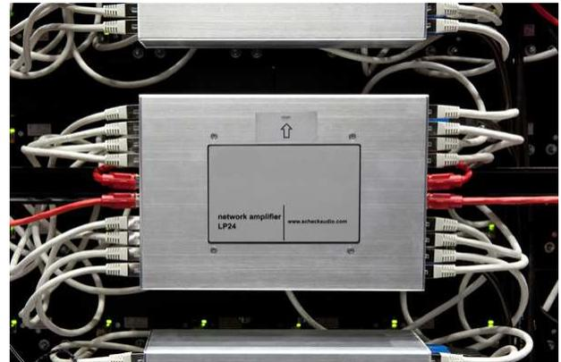
**Figure 6:** Close-up of the 16-channel network amplifier module. Grey patch cables connect the amplifier with the loudspeakers. The red patch cables are the links for the daisy chain. A green LED on the rear side of each loudspeaker indicates a proper connection.
