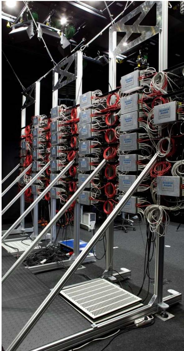
**Figure 7:** Back view of the multichannel loudspeaker system. The network amplifiers (grey boxes) are mounted directly behind the loudspeakers.
