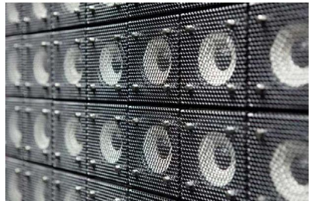
**Figure 8:** Close-up of individual speakers, arranged as a speaker wall. The interspace between the centers of two loudspeakers is 0.1 m .
